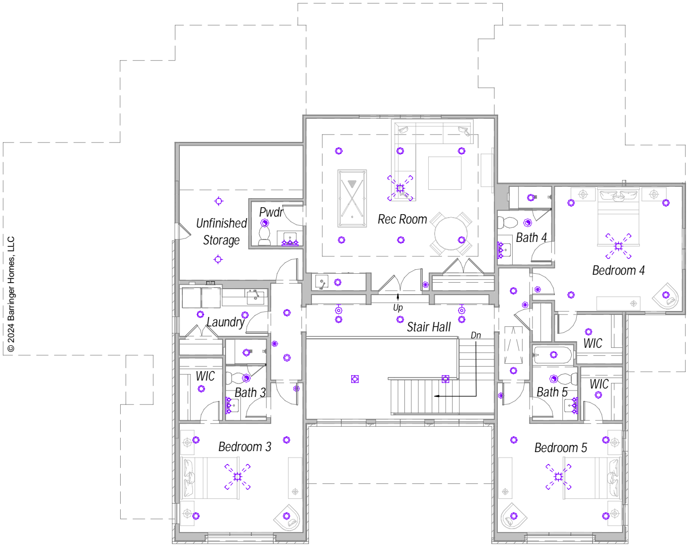
Upper Level Electrical
